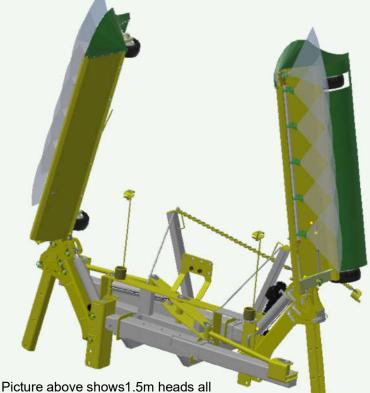
Picture above shows1.5m heads all arms fully retracted for transport, width 2.3m,
